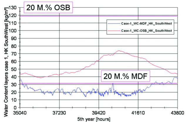
**Figure 9** WC of different layers and corresponding critical limit of 20 M%—Case 1: Holzkirchen, southwest orientation.
