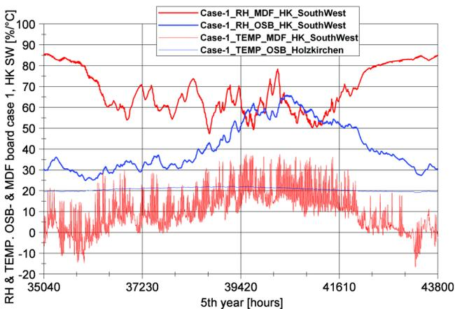
**Figure 10** RH and temperature in MDF and OSB—Case 1: Holzkirchen, southwest orientation.
