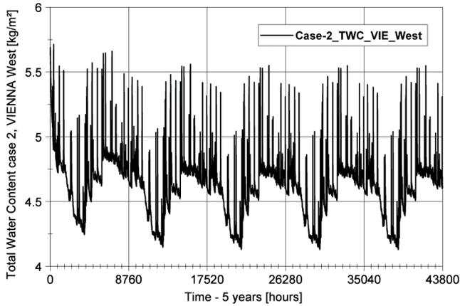
**Figure 18** Total WC wall assembly—Case 2: Vienna, west orientation.
