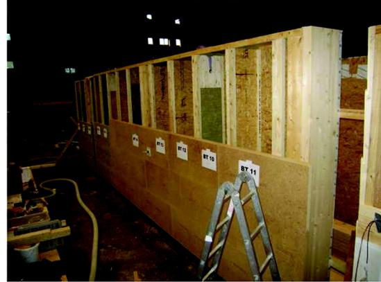
**Figure 21** Prefabricated wall assemblies and built-in measurement equipment.
