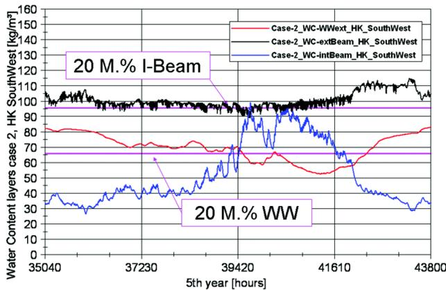
**Figure 16** WC of exterior wood-wool panel, outer I-beam area, and corresponding critical limit of 20 M%—Case 2: Holzkirchen, southwest orientation.
