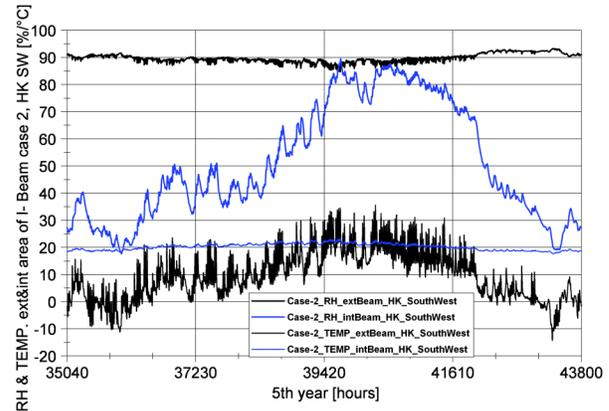
**Figure 17** RH and temperatures in the outer and inner areas of I-joint—Case 2: Holzkirchen, southwest orientation.
