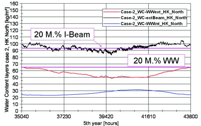
**Figure 12** WC of wood-wool panels, outer I-beam area, and corresponding critical limit of 20 M%—Case 2: Holzkirchen, north orientation.
