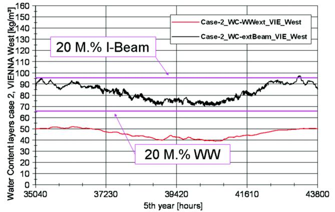
**Figure 19** WC of exterior wood-wool panel and the outer area of the I-beam and corresponding critical limit of 20 M%—Case 2: Vienna, west orientation.
