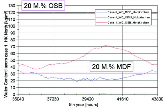
**Figure 6** WC of different layers and corresponding critical limit of 20 M%—Case 1: Holzkirchen, north orientation.
