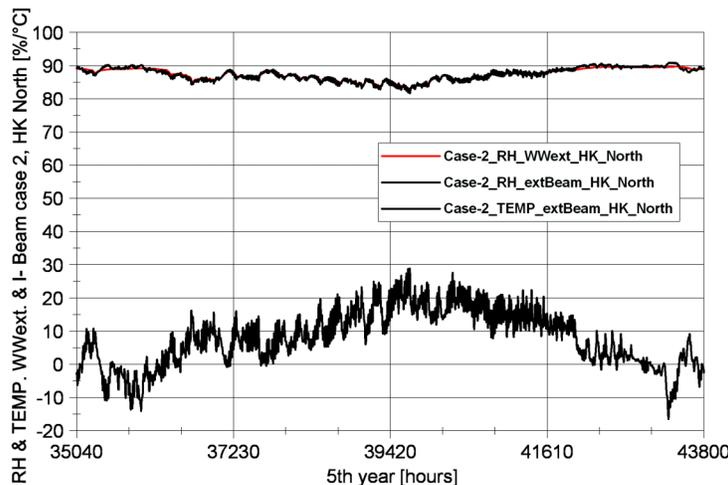
**Figure 13** RH and temperatures on the inner side of the exterior wood-wool panel and in the outer corner of the I-joist—Case 2, Holzkirchen, north orientation.
