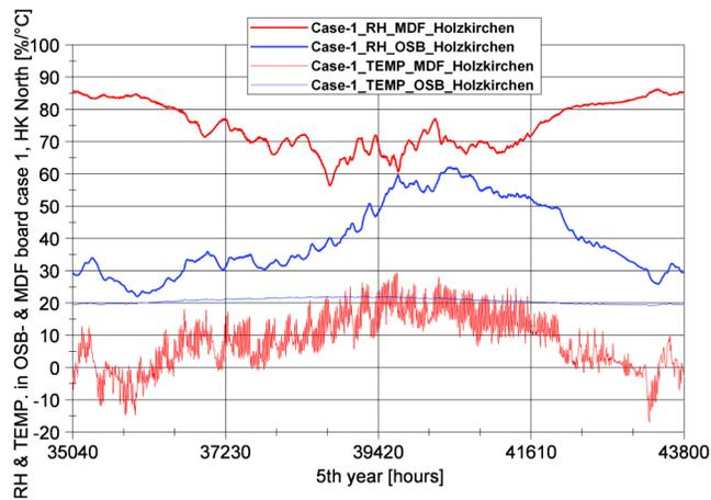
**Figure 5** RH and temperature in MDF and OSB boards—Case 1: Holzkirchen, north orientation.
